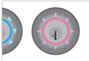
Your device is outside of activation range, the area around the lock in which it can detect your device and respond to touch. When locking or unlocking the door, bring your device closer to Kevo by turning toward the lock so that there is a direct line of sight between the lock and your device. If this happens frequently, recalibrate your device.
