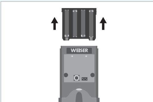
**2** Wait a few seconds, then reinsert the battery pack. The light ring will spin amber.
