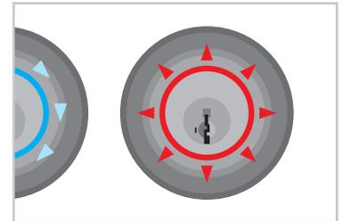
The lock has detected an unauthorized device within activation range and will not unlock. An unauthorized fob is one that has not been enrolled in your system, and an unauthorized phone is one with the Kevo app installed that does not have an eKey to your lock.
